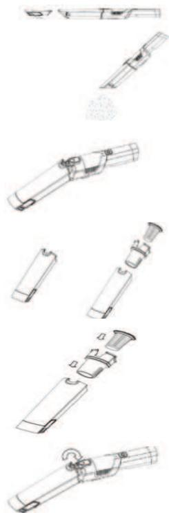
1. Press the release button (D), open the bottom cover and empty the container.
