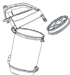
1. Press the release button and pull out the dust cup at the handle.
